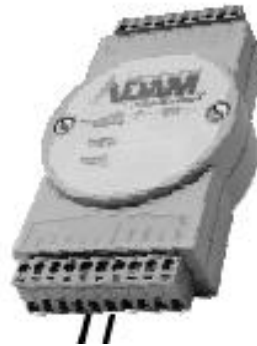
ADAM-4053, 16-Channel Digital Input Module
